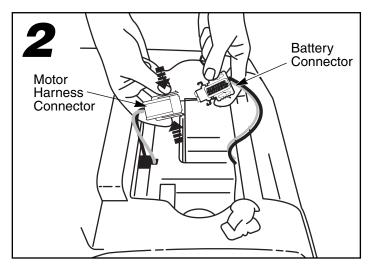
Squeeze the tabs on each side of the motor harness connector. Plug the battery connector into the motor harness connector.
